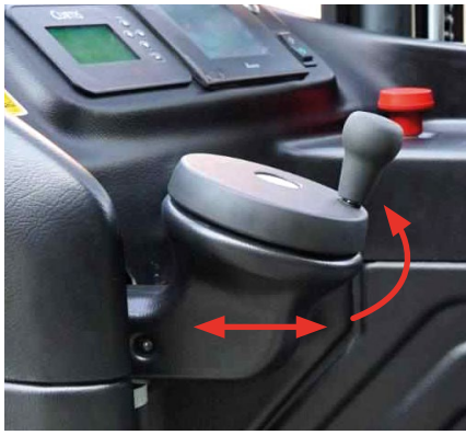
The height and depth adjustable steering wheel offers greater comfort and a better driving position.
