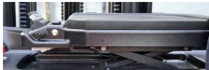
The sliding control console is adjustable in height and has a storage space.
