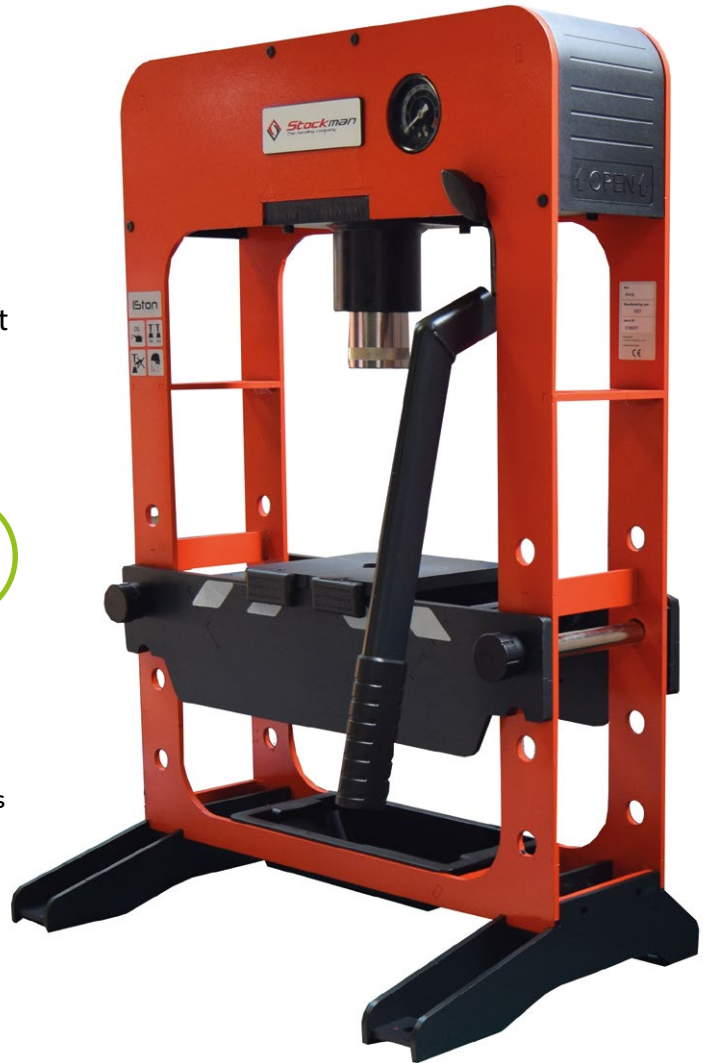
Includes a flat prism and reversible V-blocks
